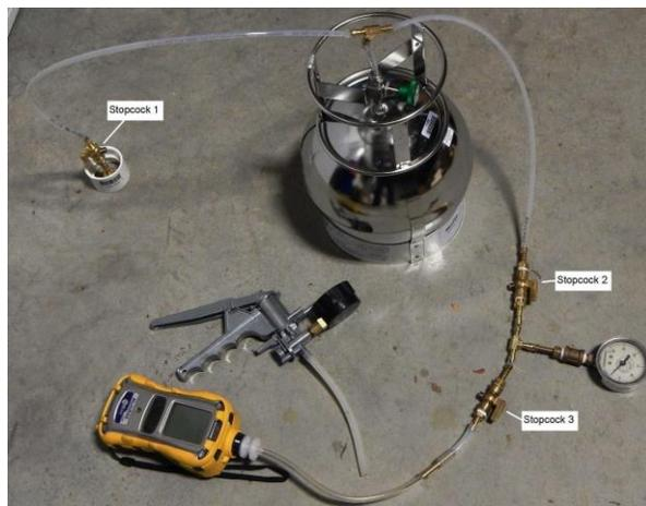
**Figure 1.** Example of Sub-Slab Sampling and Leak-Test Setup
