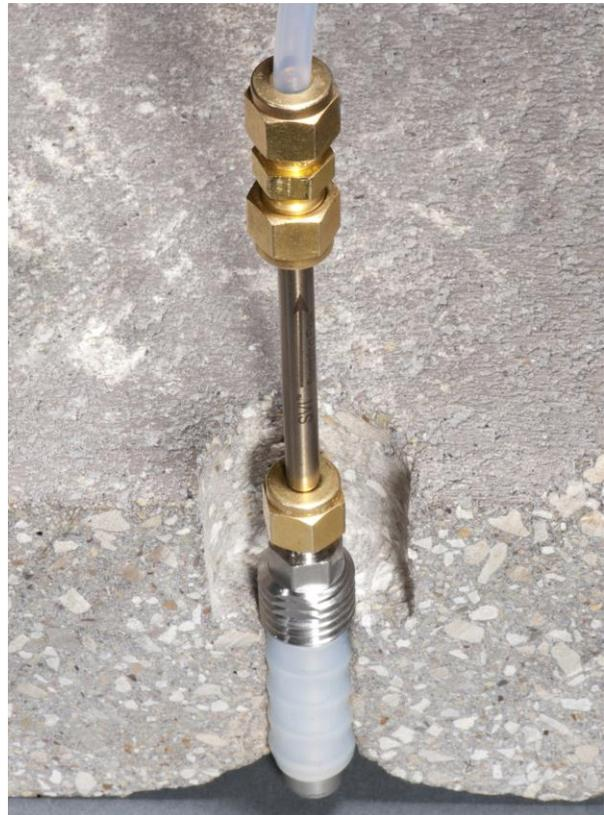
**Figure 7.** FLX-VP™ with TO-17 Sorbent tube connection
