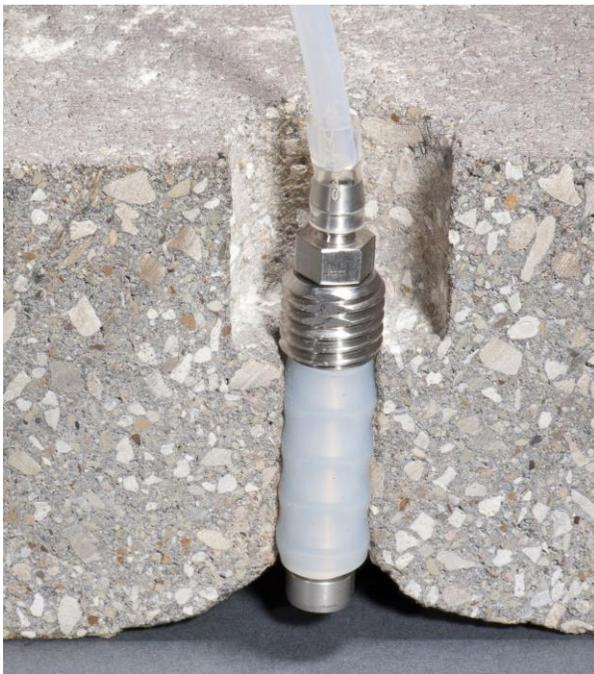
Figure 5. FLX-VP™ sample connection
