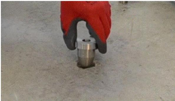
Figure 3. Testing Depth with the Drilling Guide
