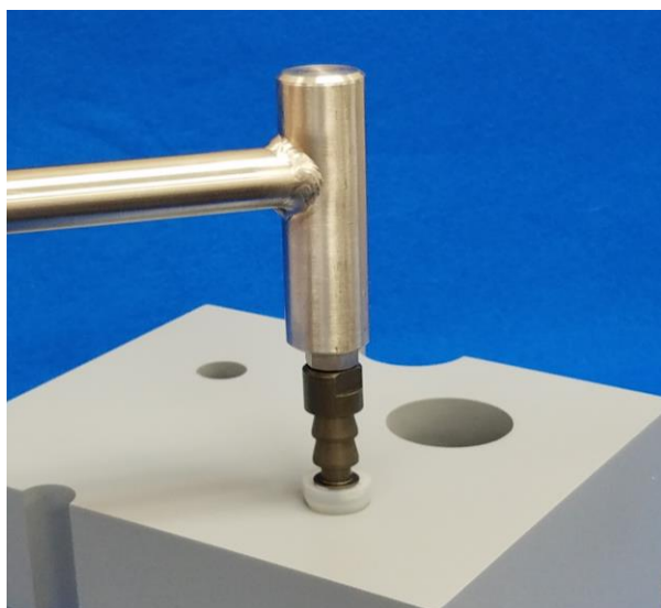
Figure 5. Mini Vapor Pin® Sampling Device Installation (Step 2)
